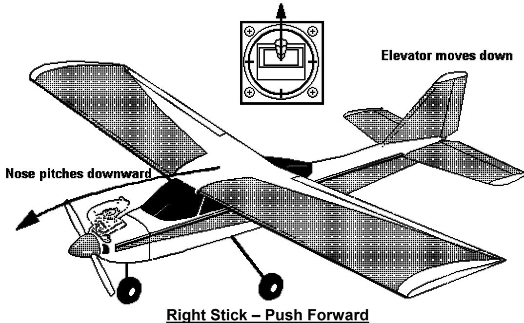
**W**hen the right stick is pushed forward, the elevator moves down. This causes the nose to pitch downward reducing the angle of attack of the wing and reducing drag. As the airplane descends its speed increases until drag and thrust are again in balance.
