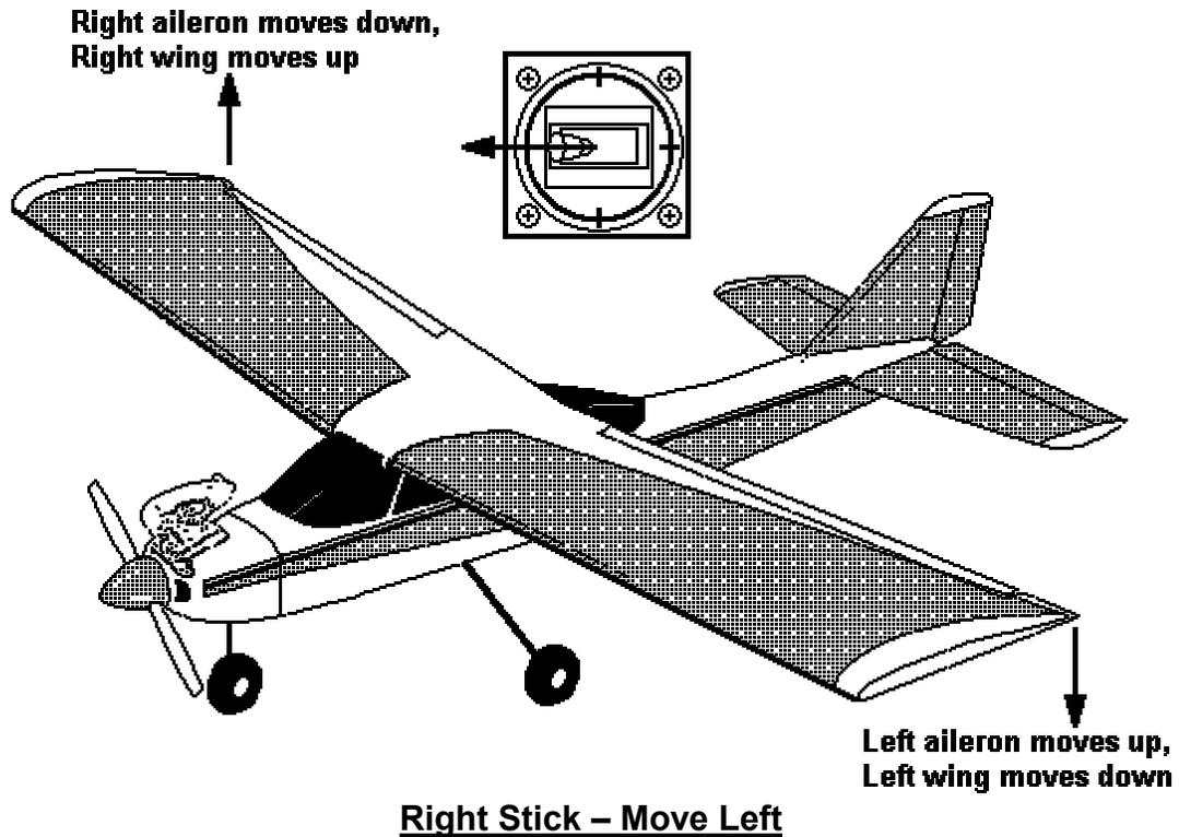
**When** the right stick is moved left, the left aileron moves up and the right aileron moves down. This causes the airplane to roll to the left meaning that the right wing moves up and the left wing moves down. It will continue to roll as long as the stick is held in the same position. When the roll takes place, lift is no longer oriented vertically so the effective lift decreases. As the angle of the roll increases, effective lift continues to decrease and the airplane will begin to drop.
