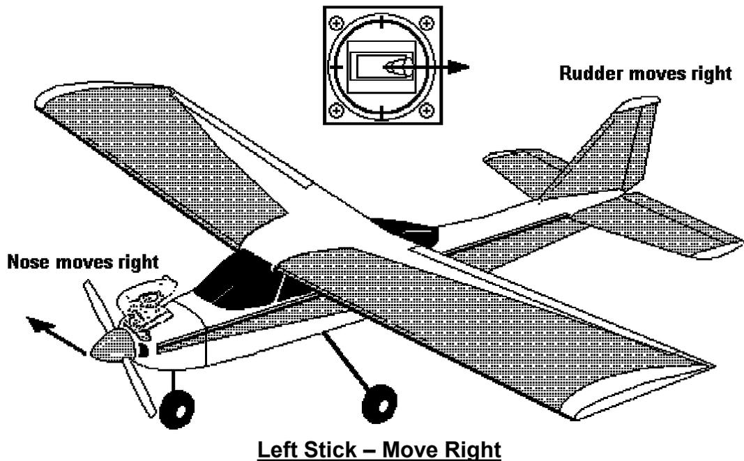
**When** the left stick is moved right, the rudder moves to the right. This causes the airplane to swing or yaw to the right. This causes the left wing to move slightly faster through the air causing an increase in lift.
