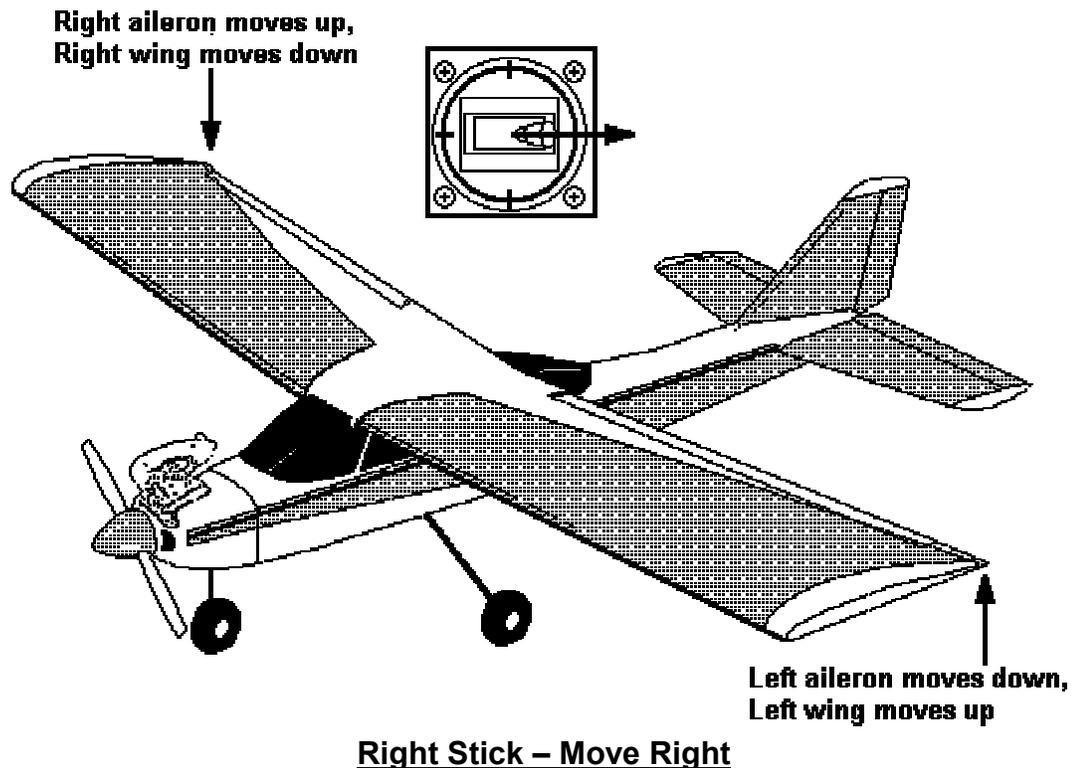
**W**hen the right stick is moved right, the left aileron moves down and the right aileron moves up. This causes the airplane to roll to the right meaning that the left wing moves up and the right wing moves down. It will continue to roll as long as the stick is held in the same position. When the roll takes place, lift is no longer oriented vertically so the effective lift decreases. As the angle of the roll increases, effective lift continues to decrease and the airplane will begin to drop.
