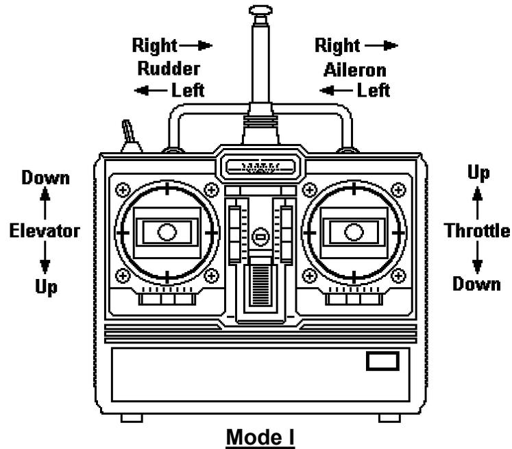
Mode I started in the days of reed actuated proportional systems. The transmitters were uniformly set up in this manner. The thought was that the elevator and rudder or ailerons were the primary controls and each should be operated by an opposite hand for precision control. Later this carried over into the more modern proportional systems since this was the mode used by most modelers.
