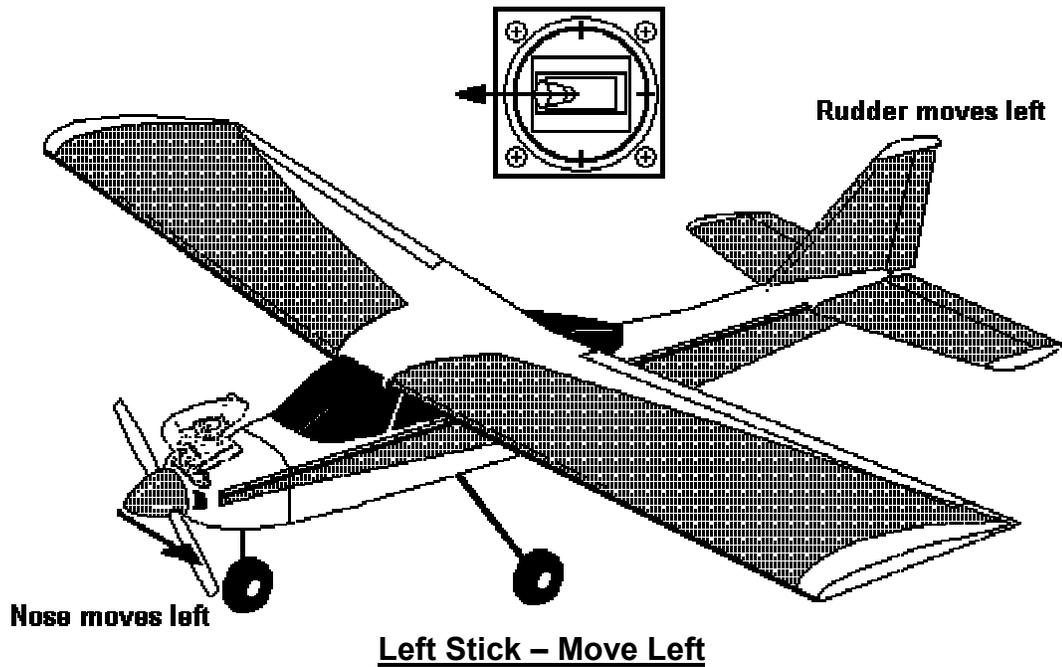
**W**hen the left stick is moved left, the rudder moves to the left. This causes the airplane to swing or yaw to the left. This causes the right wing to move slightly faster through the air causing an increase in lift. The combination of the yaw and the lift increase on the right wing results in a gentle turn to the left as long as the stick is held in position.
