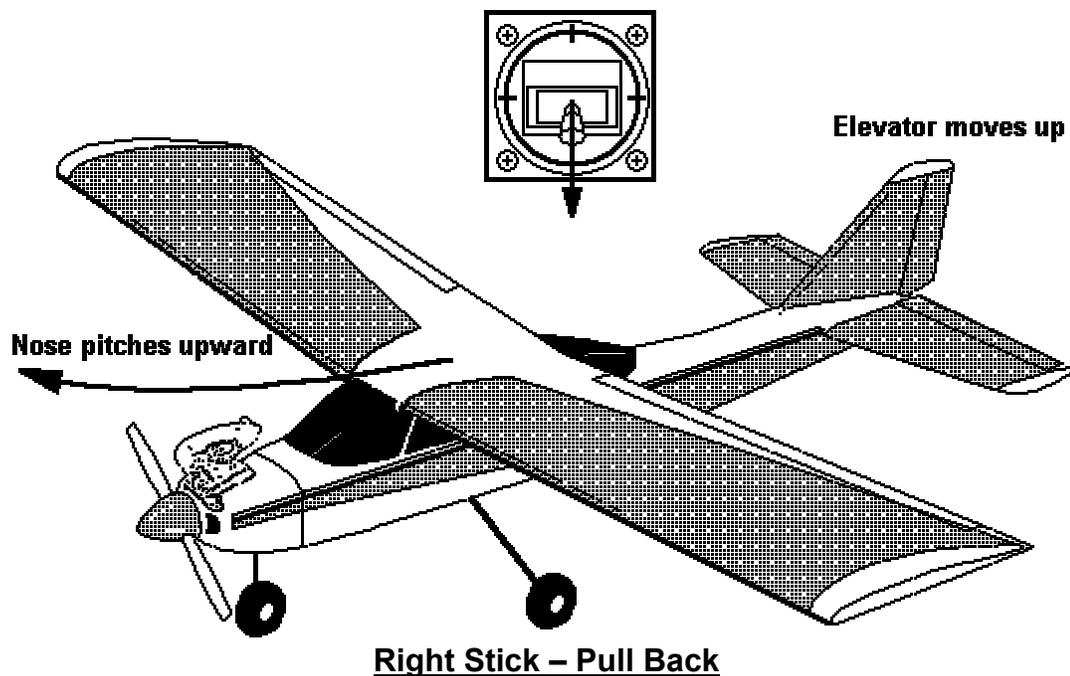
**W**hen the right stick is pulled back, the elevator moves up. This causes the nose to pitch upward increasing the angle of attack of the wing and increasing drag. If power is not applied, the airplane will slow down and eventually stall. This means that the air passing over the wing becomes turbulent and lift decreases until weight exceeds lift and the airplane will begin to drop.
