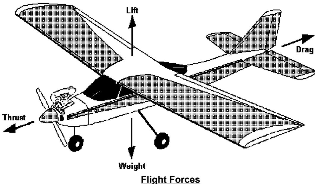
Lift increases as the velocity of the air passing over the wing increases or as the angle of attack increases as long as the flow of air over the wing remains smooth. Actual flight is attained when the force of the lift equals weight.
