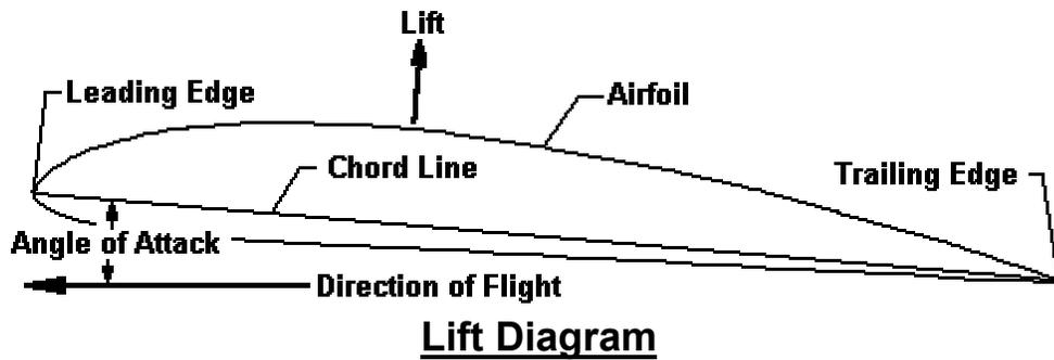
The Lift Diagram shows some of the basic terms relating to a wing section. These terms are common to R/C flight.
