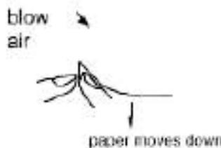
Now use your fingers to form the paper into a curve that it is slightly concave upward along its whole length and again blow along the top of this strip. The paper now bends downward.
