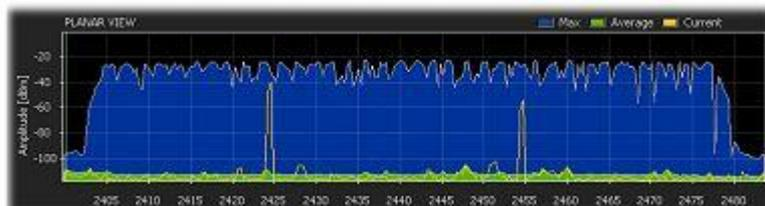
Frequency Hopping Spread Spectrum radio systems work by constantly hopping between a number of frequencies.
