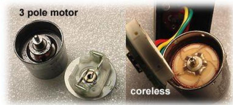
The second most common type is the coreless motor which, as the name suggests, does not have an iron-cored armature but instead has a lightweight plastic armature on which the field windings are formed. This has the advantage of being able to start and stop far more quickly (due to its low mass) and also produce more torque -- since the diameter of the windings is much greater than with a cored motor.
