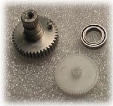
Most RC servos have a plastic case, the top section of which contains a set of gears that can be either plastic or metal. The strength and rigidity of these mechanics play a significant role in determining the robustness and weight of the servo, with metal gears usually being significantly stronger (and heavier) than plastic.
